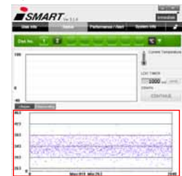
iSMART Status page can visualize how the devices utilize Wear Leveling mechanism.
