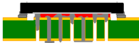
Figure 7: Solder voiding (not to scale)
